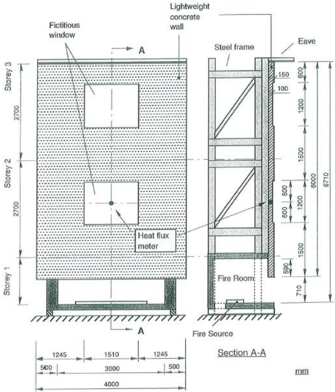
Figure 14 – SP Fire 105 Test rig (Swedish National Testing and Research Institute, 1985)
