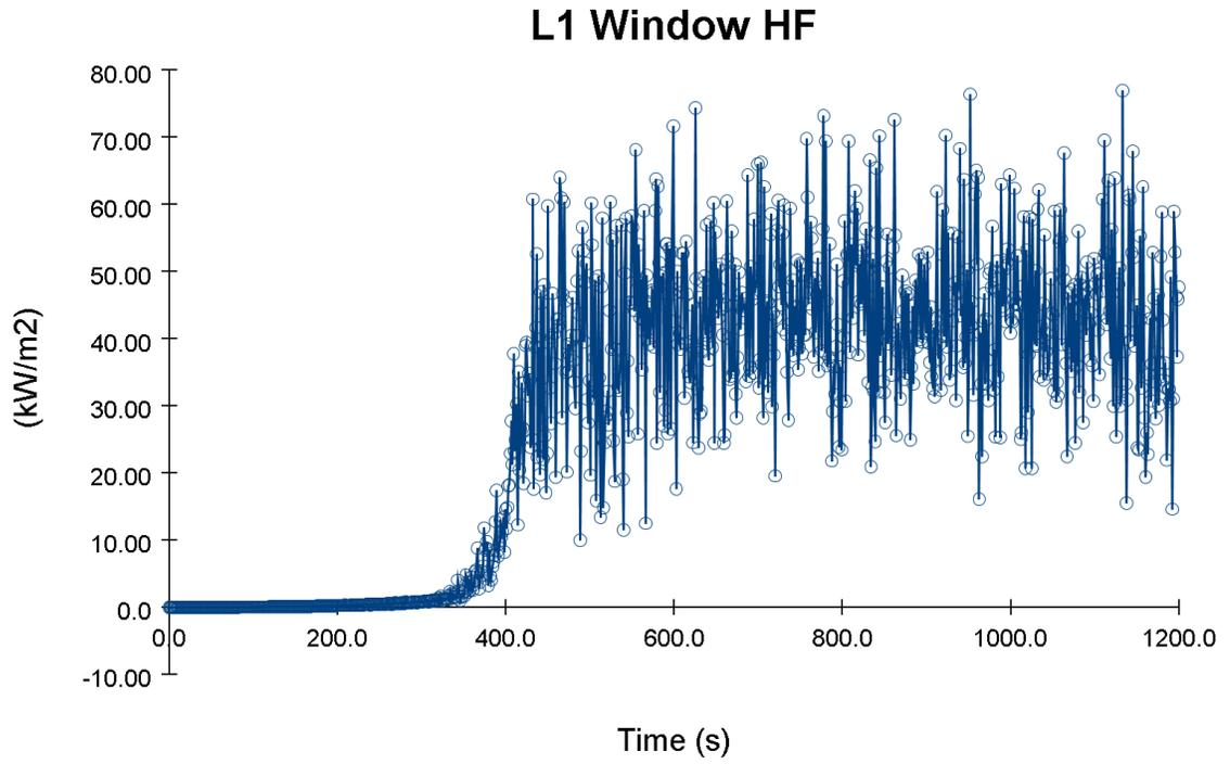
**Graph 18 – Heat flux at the window of Level 1 against time of fire**
