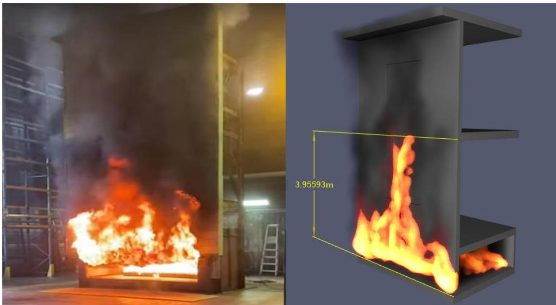
**Figure 33 – Flame height on the left of real test vs modelling simulated**
