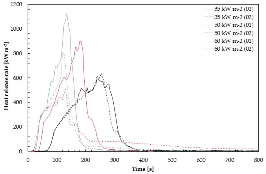
Figure 8. Heat release rate per unit area over time for samples tested with 35, 50, 60 and 80 kW m<sup>-2</sup>.
