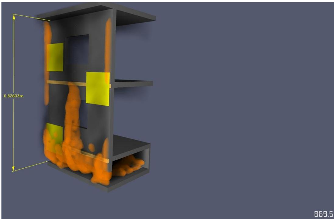
Figure 36 – Snapshot of Model 1 showing cladding burning away after 420 seconds
