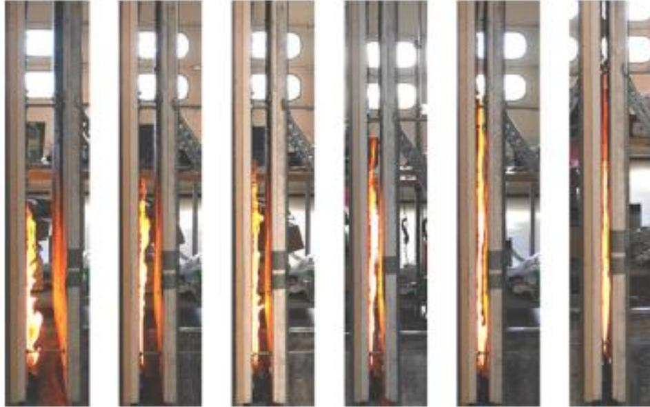
**Figure 12 – Photos of the test conducted by Karlis Livkiss showing flame height within different cavity widths**
