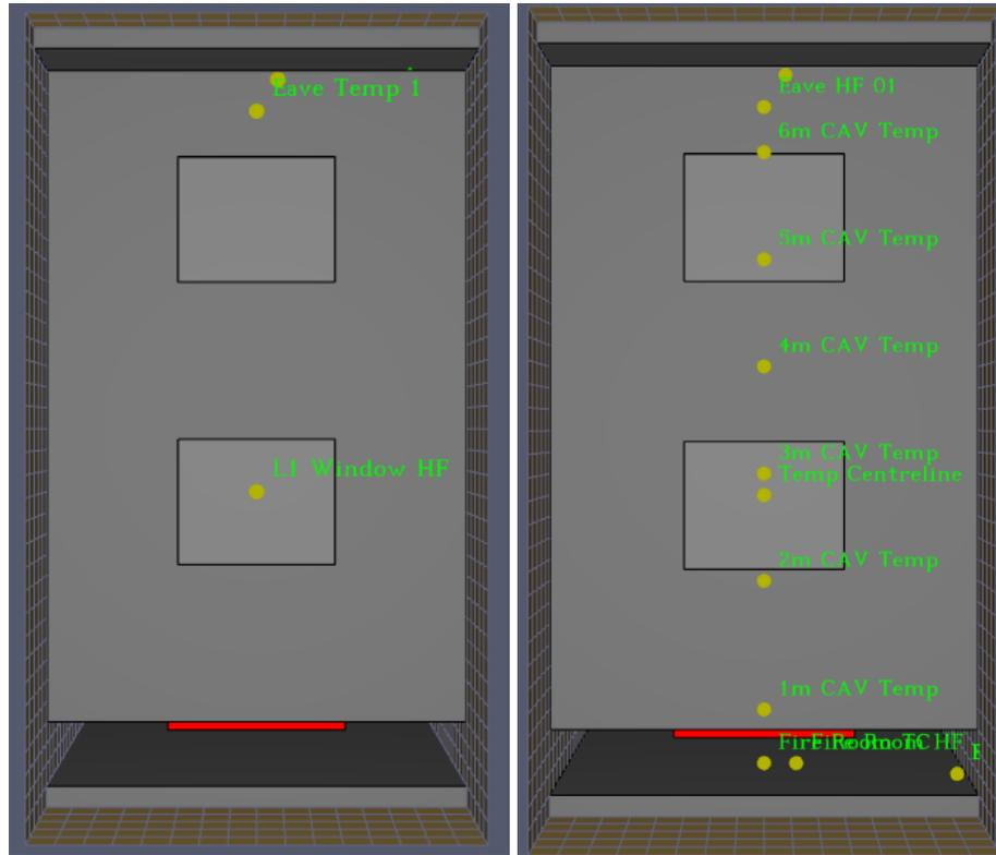
Figure 30 – Location of heat flux and thermocouple devices in the models simulated – left shows devices required by SP Fire 105, right shows additional devices placed
