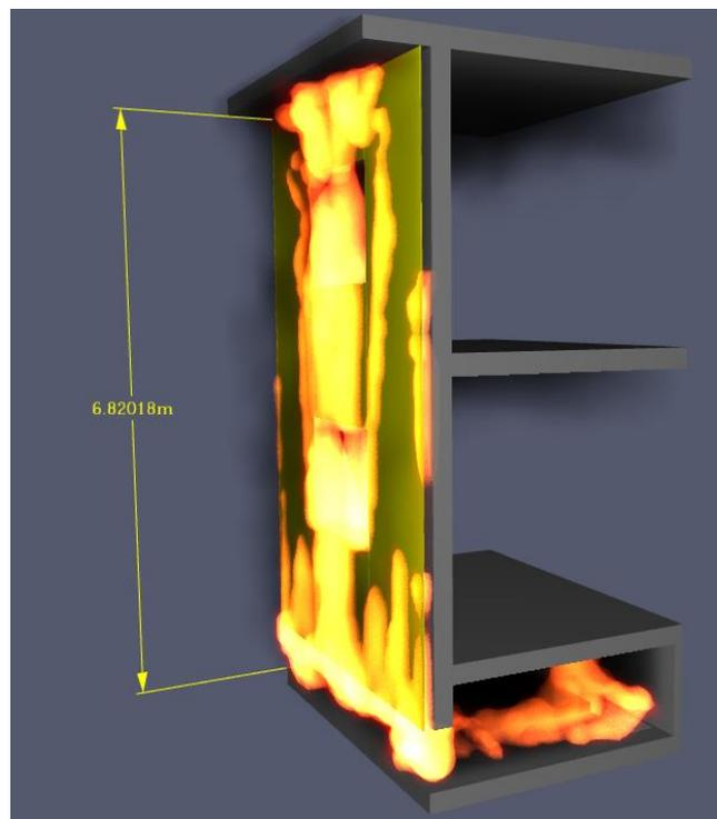
**Figure 39 – Snapshot from the modelling 2 showing height of the flame**
