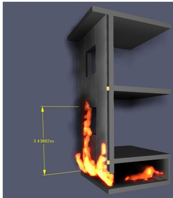
**Figure 42 – Snapshot from the modelling 3 showing height of the flame**
