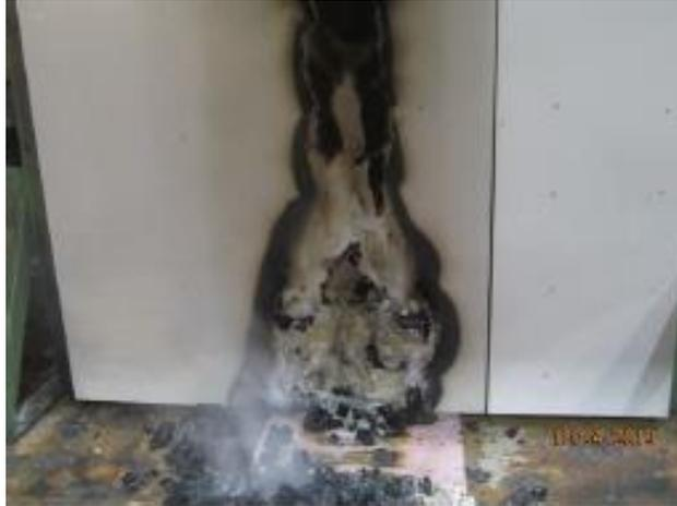
**Figure 18 – After effects of cladding after 25 minutes of 300 kW fire**
