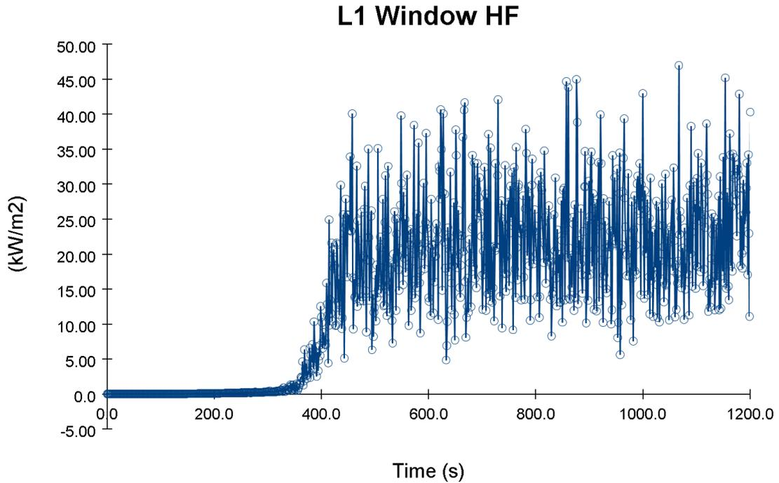
Figure 45 – Heat flux at the window of Level 1 against time of fire
