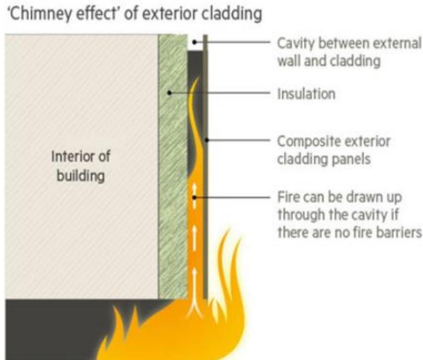
**Figure 1 – A building façade system with a cavity as a possible route for fire spread.**
