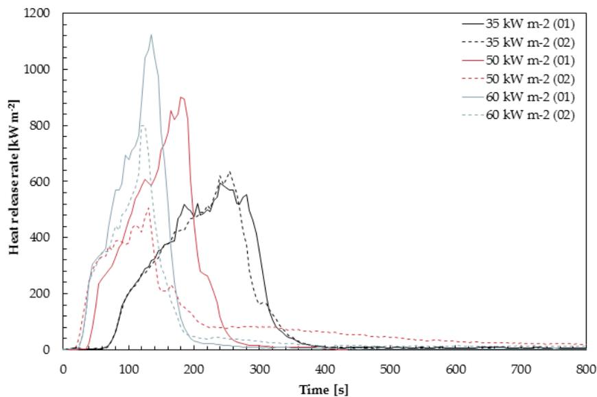
**Graph 2 – Heat release rate per unit area over time for samples tested at different heat fluxes**
