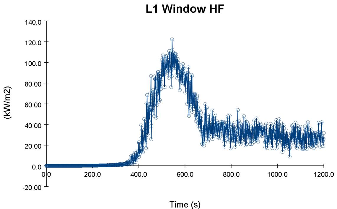
**Graph 14 – Heat flux at the window of Level 1 against time of fire**
