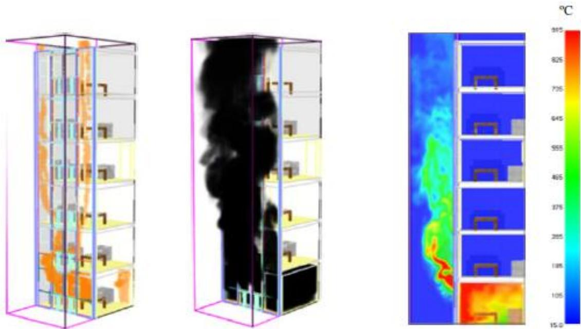
**Figure 13 – Extract from the modeling conducted by (Giraldo, et al., 2013), showing the spread of fire and smoke through the cavity and building façade from a room fire**
