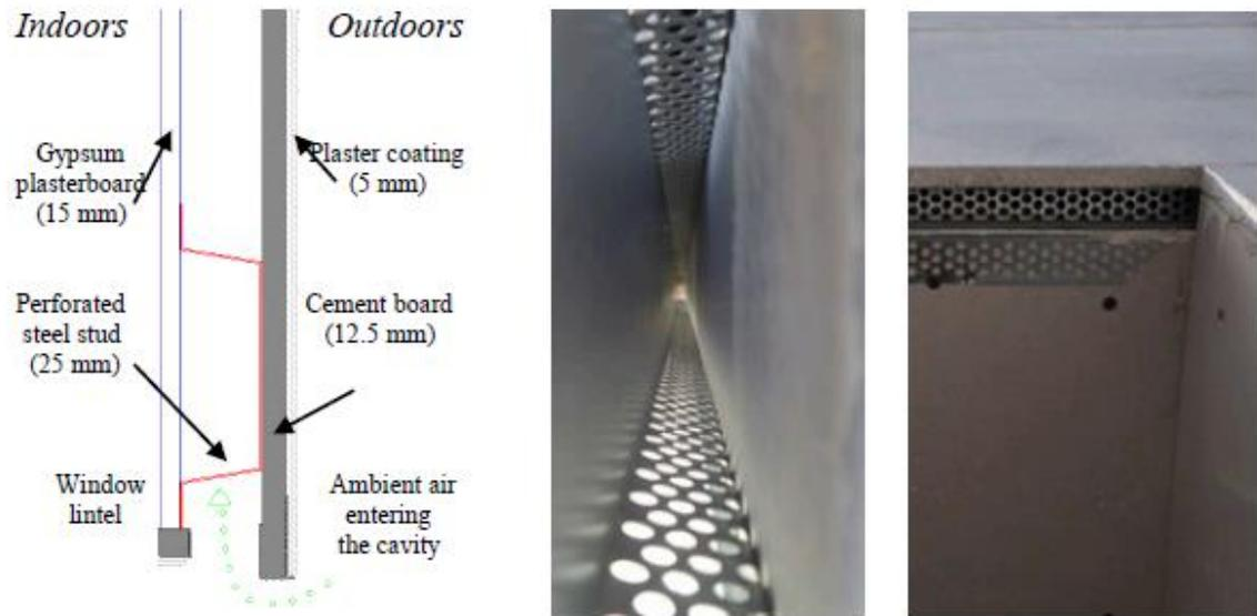
**Figure 11 – Extract taken from the research paper conducted by Kolaitis 2014, showing Ventilated Façade System build up**
