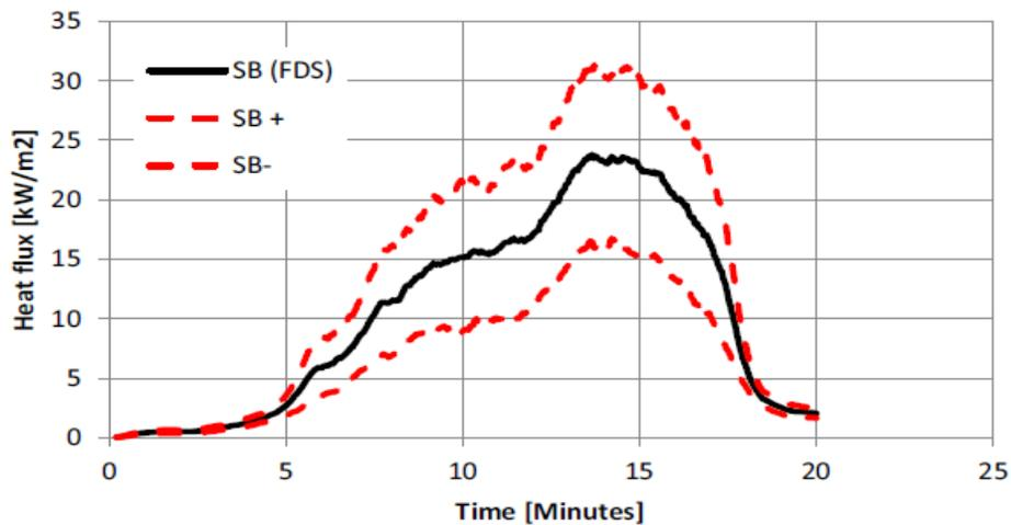
**Graph 7 – Heat flux achieved at the center of the fictitious window taken from the validation SP Fire 105 test paper**
