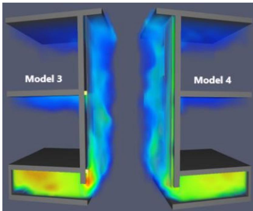
**Figure 48 – Thermographic comparison between Model 3 & 4 showing cavity temperature**
