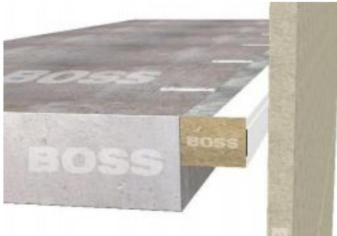
**Figure 8 – Rockwool based product with intumescent strip at the end which expands upon reaction with heat (approx. 150 degrees C) to seal the cavity**
