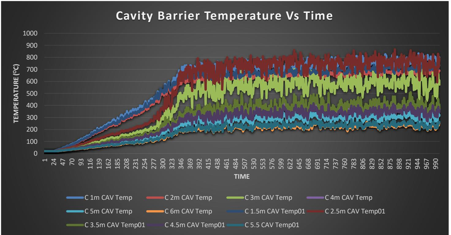
**Graph 17 – Graph showing temperature of the cavity at different heights of Model 4**
