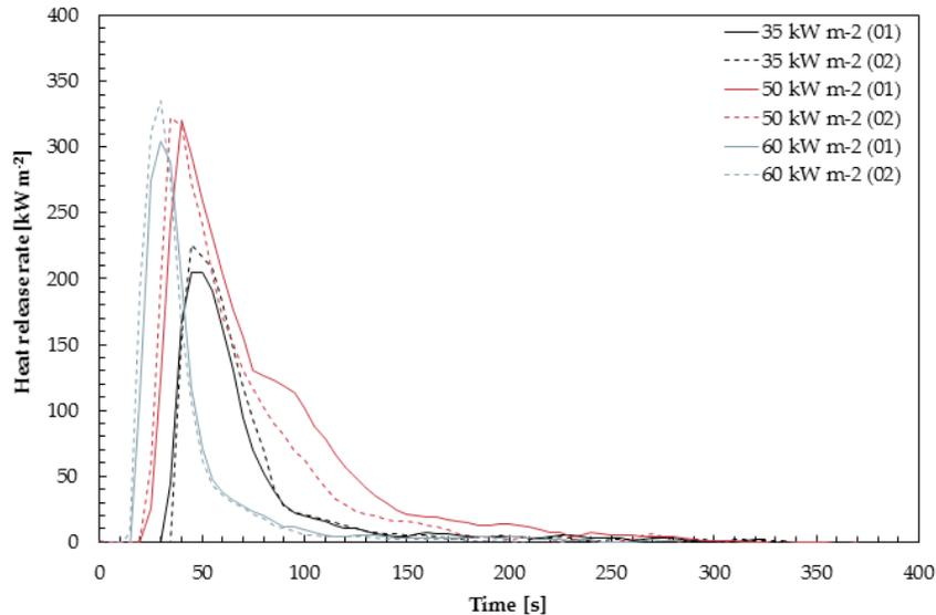
**Graph 3 – Heat release rate per unit area over time for samples tested at different heat fluxes**
