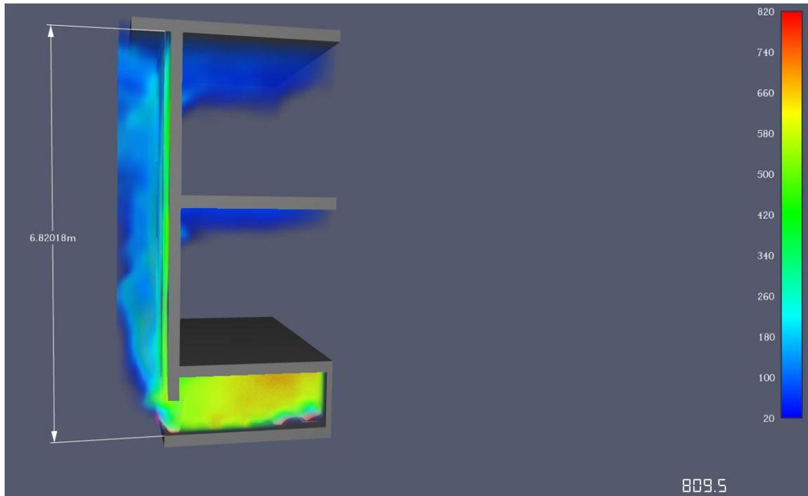
**Figure 47 – Snapshot of Model 3 thermographic showing maximum temperature reached**
