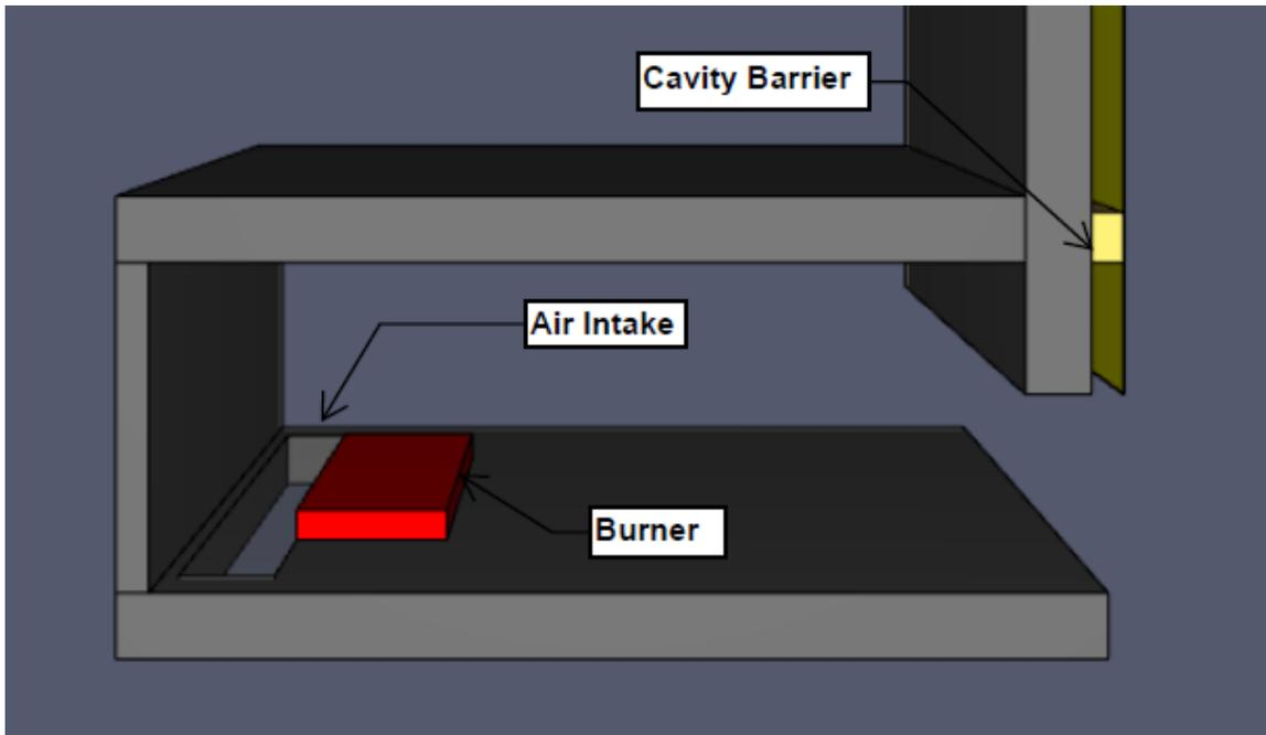
**Figure 29 – Cavity barrier used in Model 1 and Model 3**
