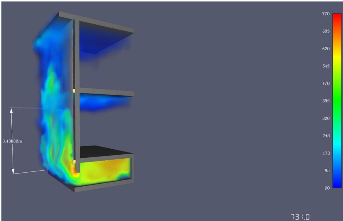
**Figure 44 – Snapshot of Model 3 thermographic showing maximum temperature reached**
