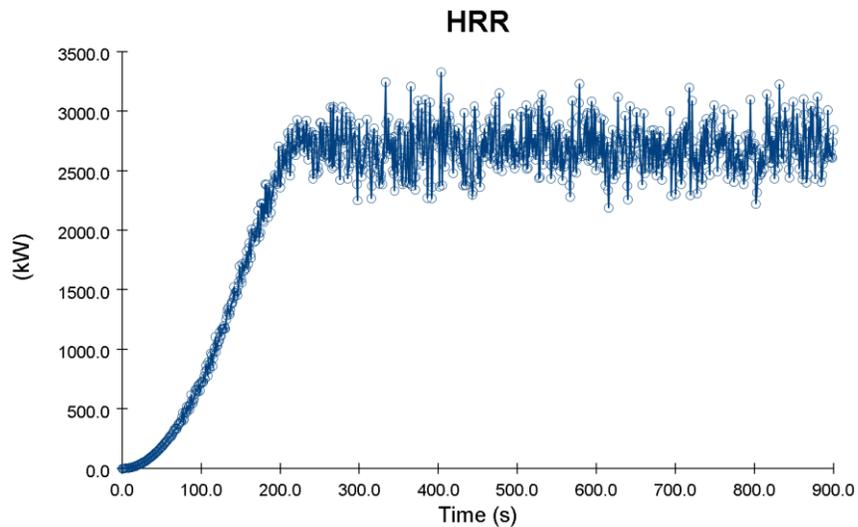
**Graph 5 – Heat release rate of the fire from the base model conducted**
