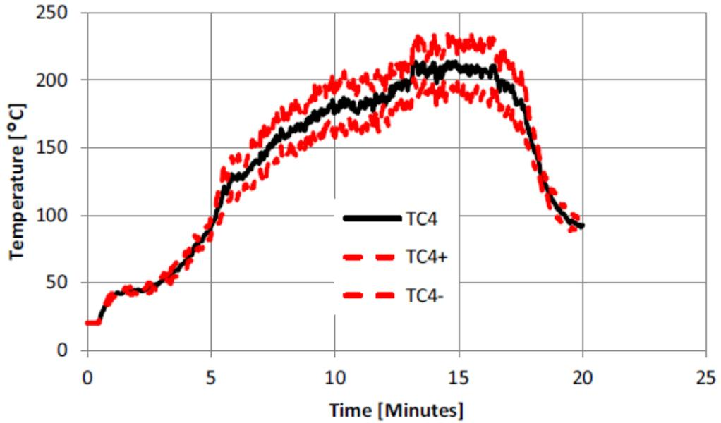
**Graph 9 – Temperature of the eave thermal couples taken from the validation SP Fire 105 test**
