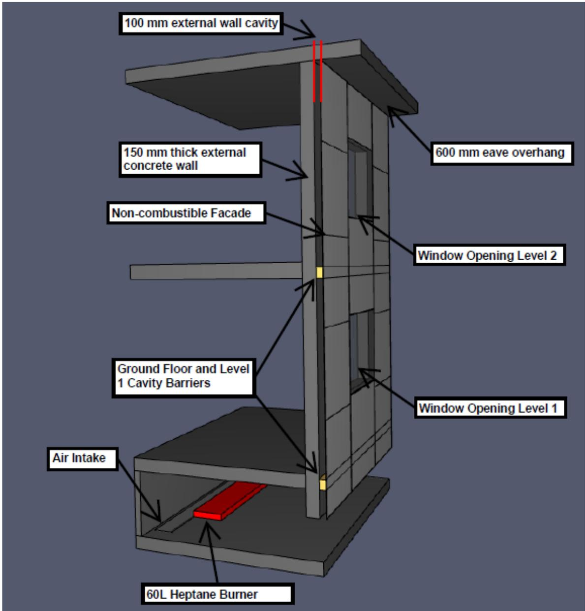
Figure 23 – Snapshot of Model 3 from the FDS modelling done
