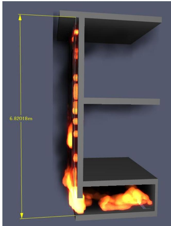
**Figure 46 – Snapshot from the modelling 3 showing height of the flame**
