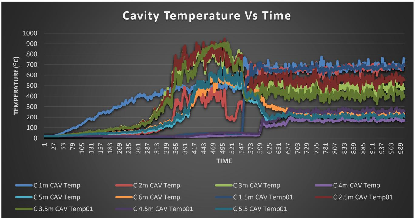
**Graph 12 – Graph showing temperature of the cavity at different heights of Model 1**
