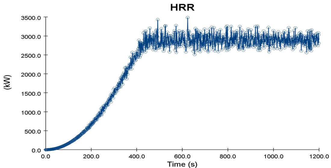
Figure 43 – Graph showing heat release rate of the fire of Model 3
