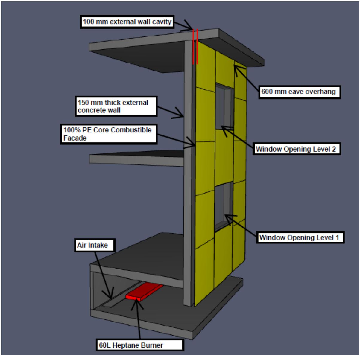
Figure 22 – Snapshot of Model 2 from the FDS modelling done
