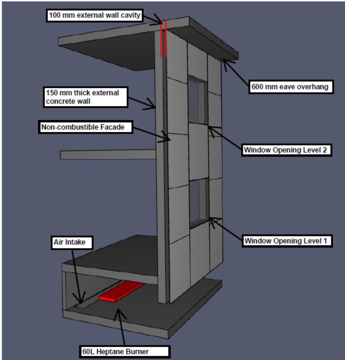
Figure 24 – Snapshot of Model 4 from the FDS modelling done
