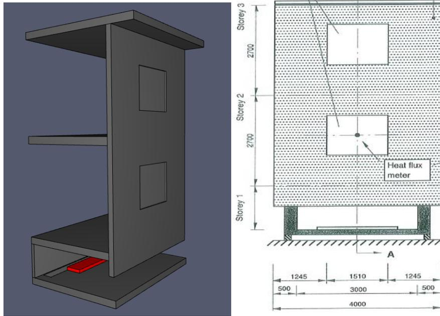
Figure 27 – Rig Dimensions based on SP Fire 105 Test
