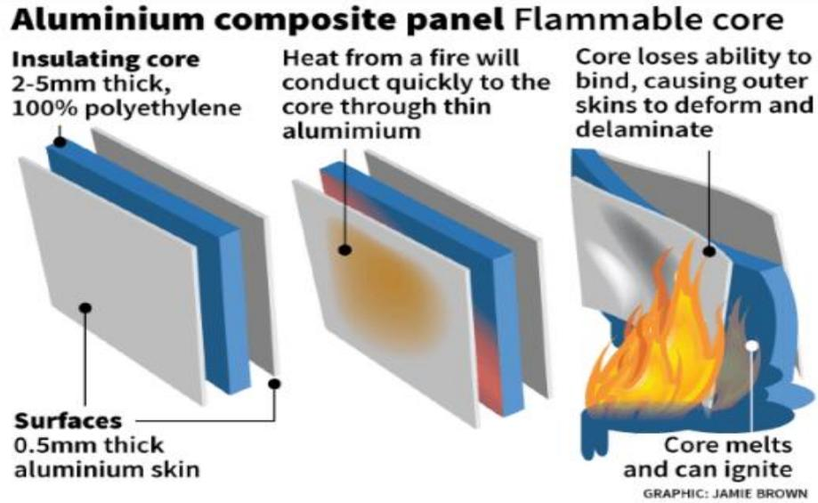
Figure 3 – Figure showing ACP make-up and how fire impacts on its performance (al, 2020)
