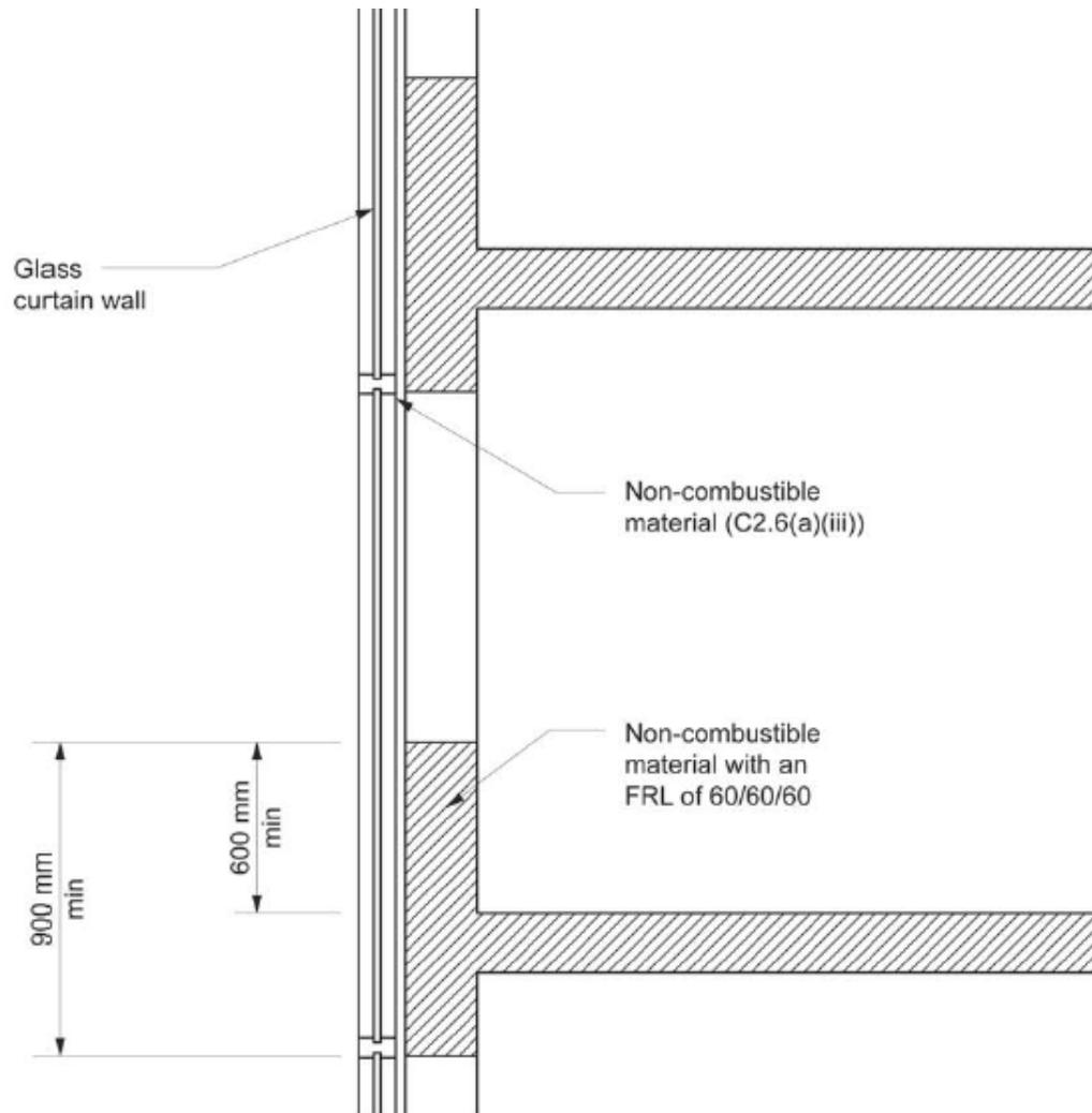
**Figure 4 – Extract of the Guide to NCC 2019 from Clause C2.6, showing detail of vertical fire separation along a curtain glazed wall with a cavity**
