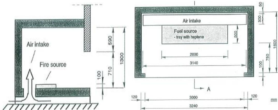
**Figure 26 – Extract from the SP Fire 105 Test showing fire source and air intake (Swedish National Testing and Research Institute, 1985)**
