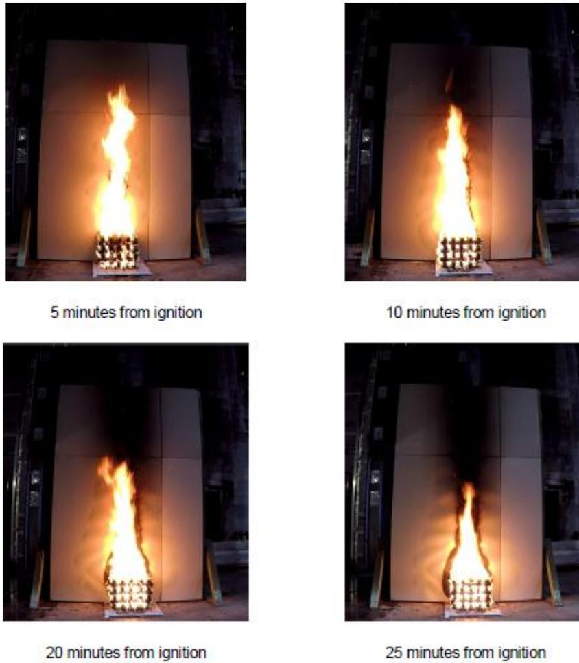
Figure 17 – Intermediate fire test on A2 ACM showing results after 25 minutes
