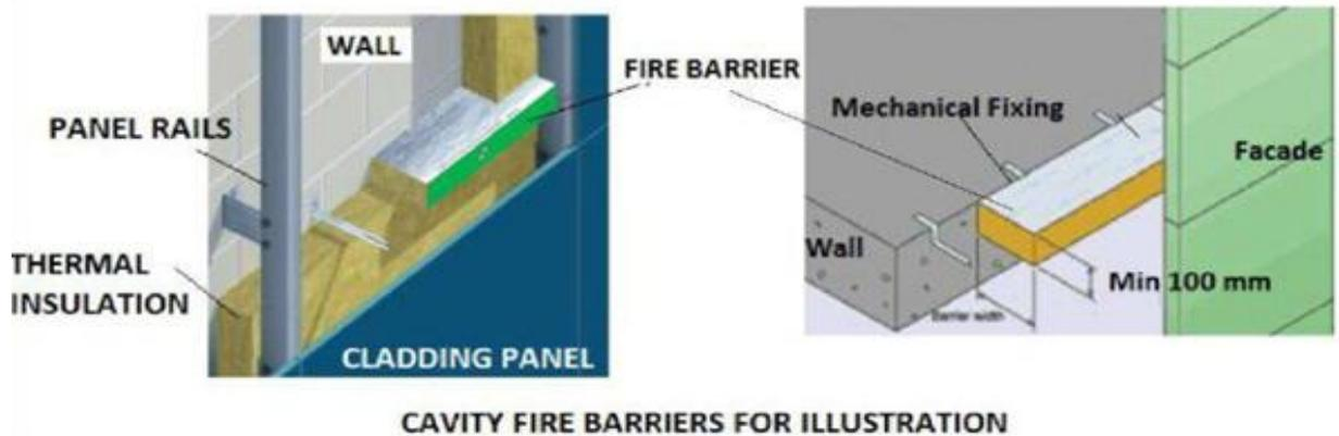
Figure 10 – Section 4.5.4 of the UAE Code describing relevant requirements for cavity barriers
