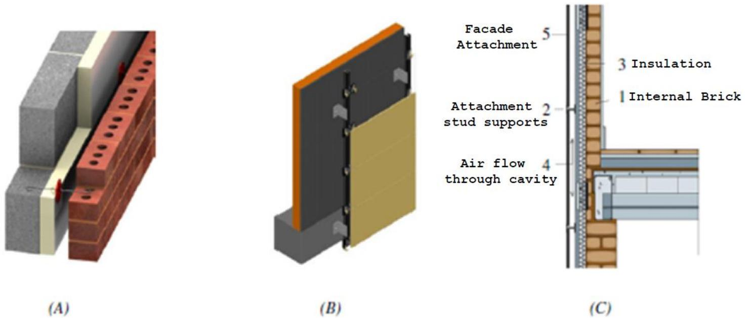
**Figure 5 – Façade cavity systems (A) Cavity wall (B) Ventilated façade (C) elements of ventilated façade** (Giraldo, et al., 2013)
