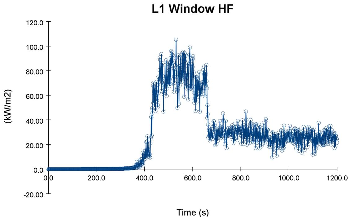
Figure 38 – Heat flux at the window of Level 1 against time of fire
