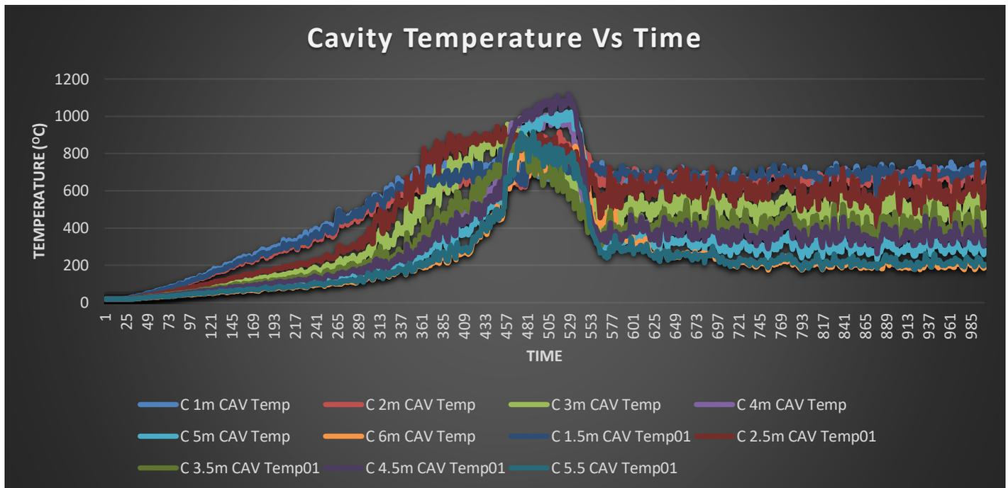
**Graph 13 – Graph showing temperature of the cavity at different heights of Model 2**
