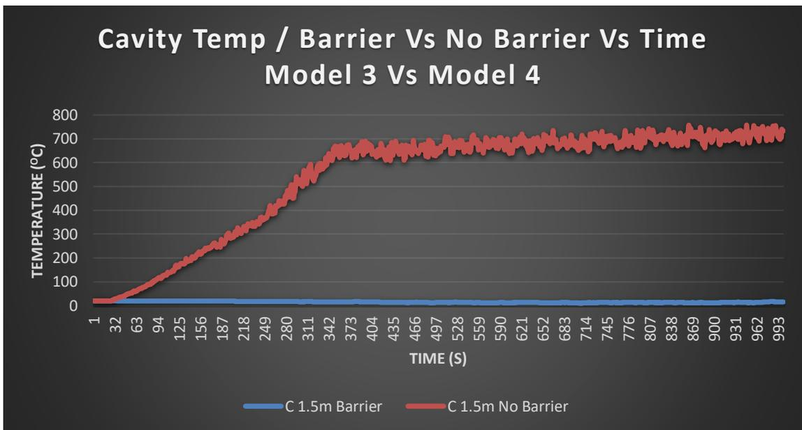
**Graph 20 – Cavity temp at 1.5 m shown for model 3 & 4 (barrier Vs no barrier, non-combustible)**
