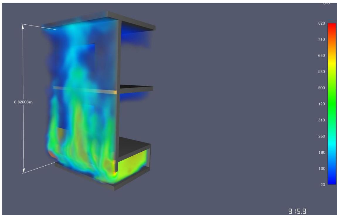
**Figure 37 – Snapshot of Model 1 thermographic showing maximum temperature reached**
