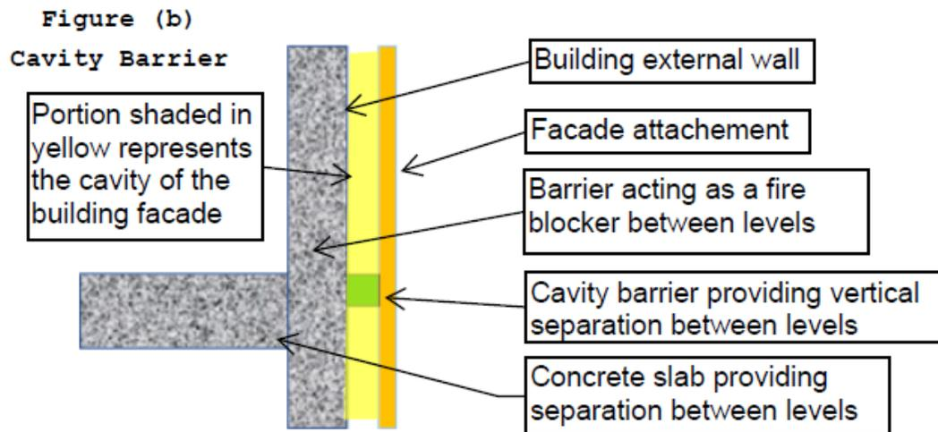
**Figure 6 – Caption showing elements of (a) perimeter fire stopping installation; and (b) cavity barrier installation**
