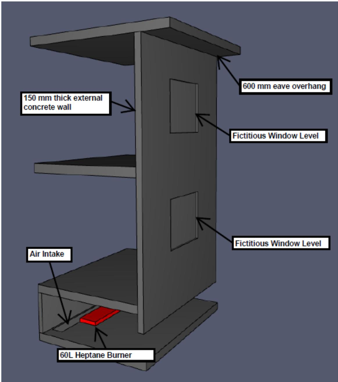
Figure 20 – Base model replicating SP Fire 105 test
