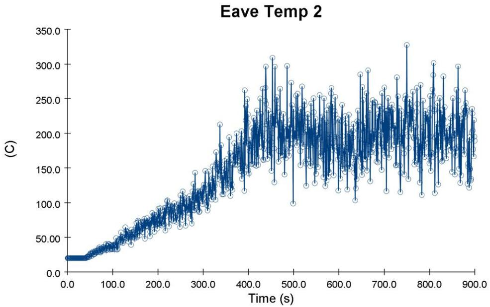
Graph 8 – Graph showing temperature of the thermocouples located directly below the eaves
