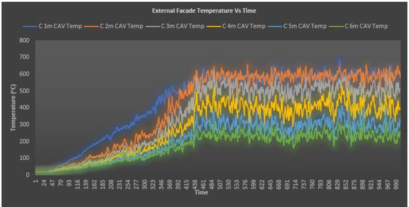
**Graph 10 – External façade temperature of the Base Model shown at every 1m up to 6m at 900 s**
