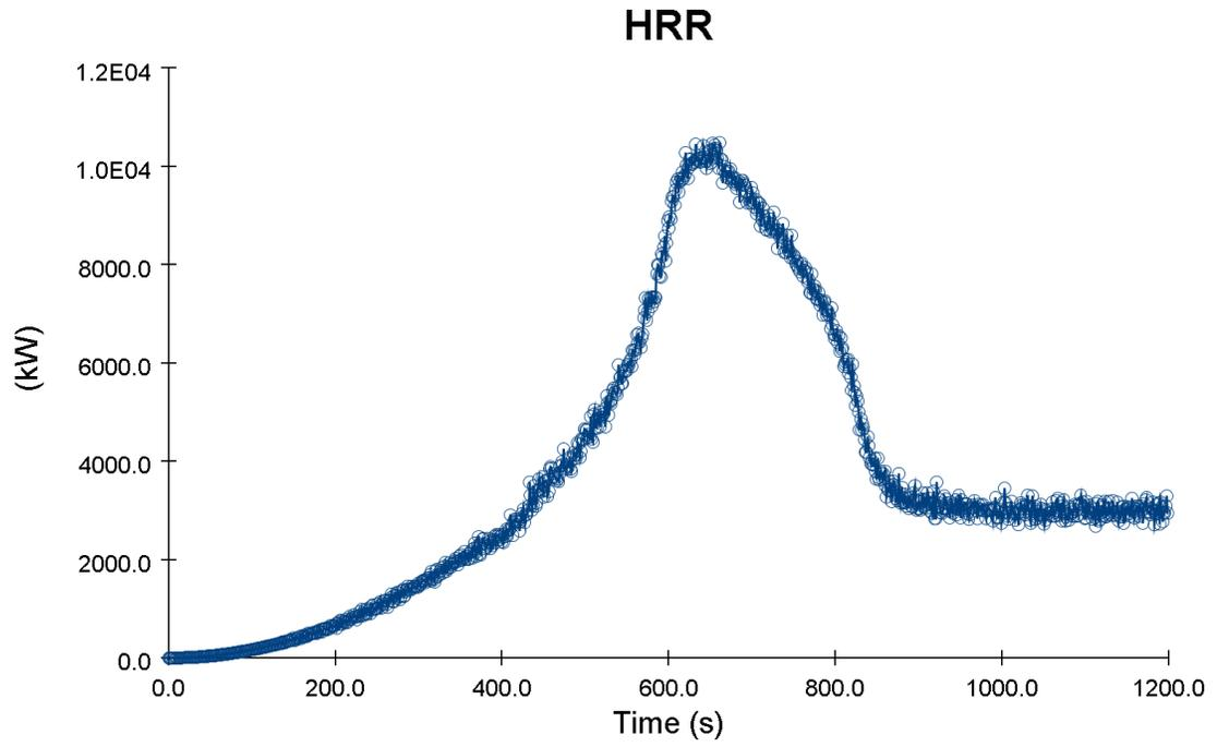
Graph 11 – Graph showing heat release rate of the fire
