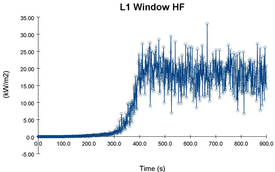
**Graph 6 – Heat flux at the window of Level 1 against time of fire**
