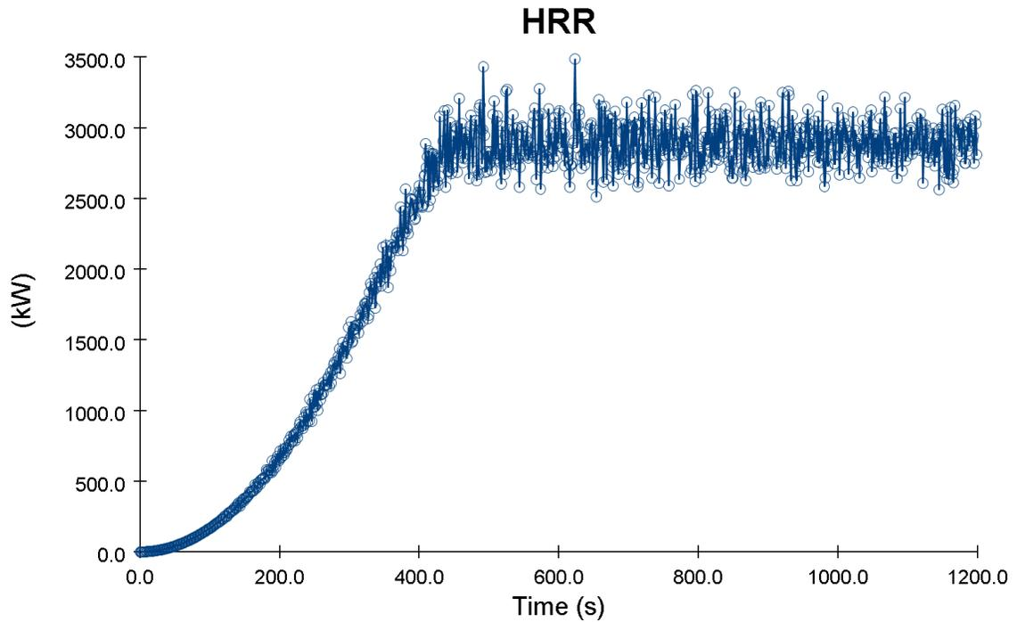
**Graph 16 – Graph showing heat release rate of the fire of Model 3**
