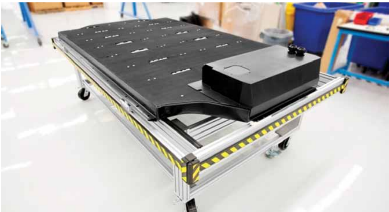
Below: Figure 7, Tesla Model S lithium-ion battery pack 9
